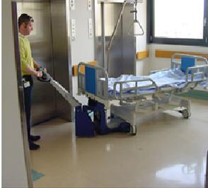
Professional pedestrian operated electric vehicle with tiller head system, suitable to move hospital beds, x-ray trolleys, laundry carts, and/or medical waste trolleys up to 350 Kg.
